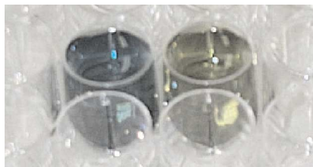
Figure 6. A microtiter well (right) that contains cAMP (500 \mu\text{M} ), PDEs (0.023 \mu\text{M/L} ), the sensor (50 \mu\text{M} ) and IBMX (500 \mu\text{M} ) is colored blue but the well (left) that contains the same mixture except IBMX is yellow. The picture was taken after incubating the mixture for 1 h at room temperature.
